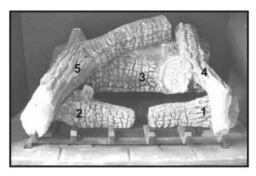
**STEP 6:** (SRV2057-724): Notch in left end of Log 5 will interlock with front left corner of grate. Rest right end of log so that it engages tab on log 3. Log 2 may need to shift to right slightly.
